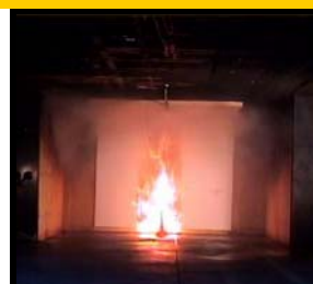
22 Seconds— Sprinkler Operates
